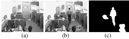
Fig. 1. Example of target detection: (a) background, (b) foreground, and (c) detection result
